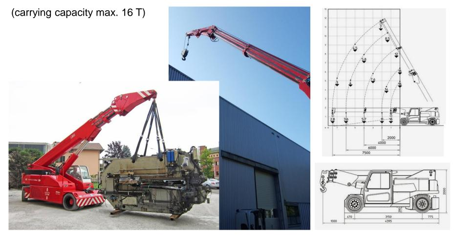
**Capabilities cabin-controlled portable crane**
